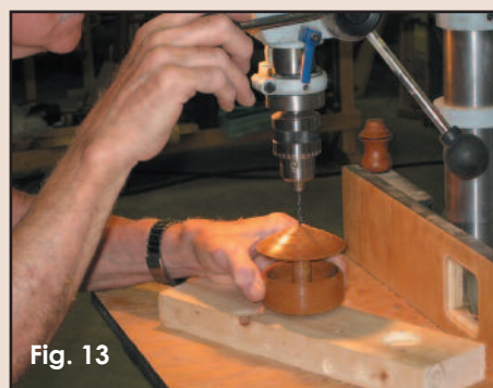
Fig. 13 Drill a hole for the screw eye on the drill press.
