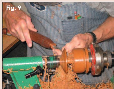
Fig. 9 Switch to the angled scraper to refine the moat area.
