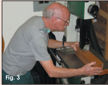
Fig. 3 Cut the blank to length on the bandsaw.
