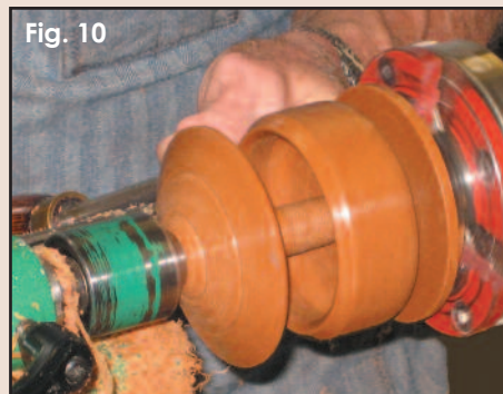
Fig. 10 Form the bottom with the 3/8" gouge.
