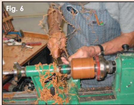
Fig. 6 Start to cut the taper for the roof.
