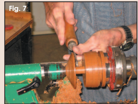
Fig. 7 Turn the stem down to 3/4" diameter.
