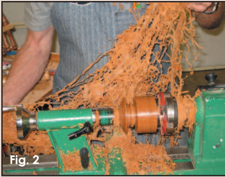
Fig. 2 The material will come off the tool in long ribbons that could get tangled in the lathe; so use caution and stop often to clear away the waste.
