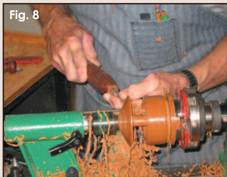
Fig. 8 Start to remove excess material with the scraper.
