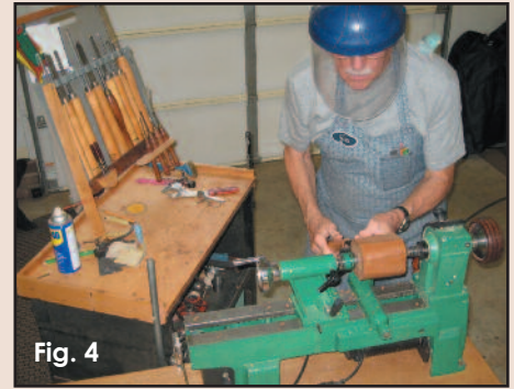
Fig. 4 Turn the blank to a cylinder first.
