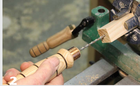
2 Drill a hole through the blank.
