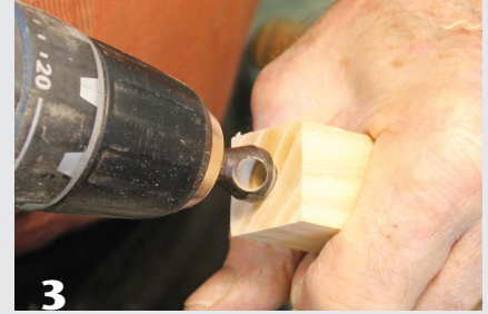
3 Countersink both ends of the blank.
