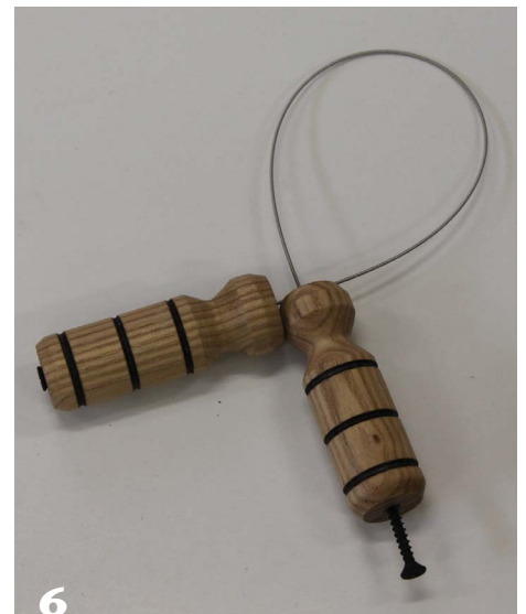
6 Affix the wire to the handles using drywall screws. The wire is inserted through the top all the way to the bottom of the handle, where the drywall screw pinches it firmly in place. Note the screw at right is left unfastened for the purpose of illustrating the tool's construction. Tighten both screws to hold the wire firmly in place prior to using the tool.
