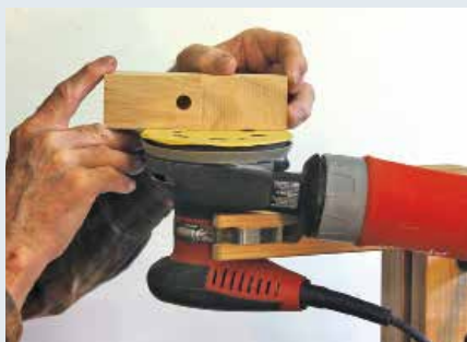
On top sanding made very easy
