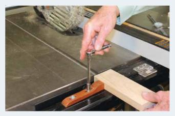
3. Drill the clamping bar and mount the gauge with screws in the middle of the slots. Take the previously cut piece and hold it against the fence bar, bring up the gauge so that it is just snug and tighten the mounting screws. This gauge is now set.
