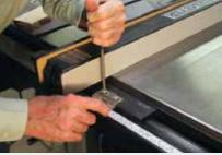
3. Then from this dimension adjust the rip fence gauge to read the same measurement on the clamping bar rule. Lock the fence gauge in place. With this small adjustment you have eliminated measuring from the tip of one tooth to the side of the rip fence and then having to make multiple test cuts to get it perfect. Speed and accuracy improve along with the ability to use other jigs, as you will see later on.
