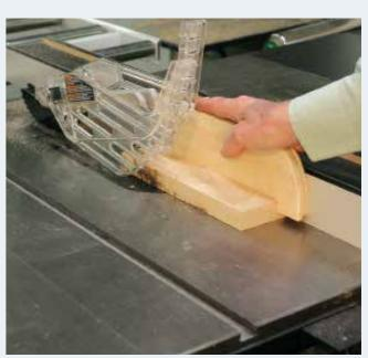
2. Next, take a piece of hardwood scrap jointed on one side and make a cut about 50mm wide. Do NOT move the rip fence. Take the cut piece and place it at the end of the rip fence clamp and hold the new gauge against it. Locate and drill two holes in the clamping bar for the metal screws.
