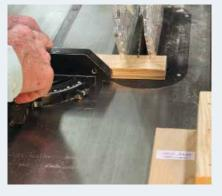
5. ... extend the piece to the new gauge and make a cut. Repeat this to cut a second piece and then as many more as you like.
