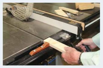
4. To give it a try, move the rip fence away. Take a scrap piece of wood you would like to duplicate the width of, place it against the gauge and bring the ripsaw fence up to it. Lock the fence in place.
