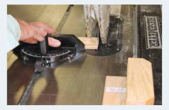
3. Next, with the use of the crosscut gauge, make a small cut to square and clean up the end of the board.
