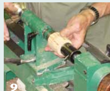
9 Glue and clamp two discs together using the tailstock to apply pressure.
