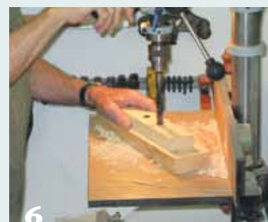
6 After drawing a series of circles onto a length of hardwood, drill holes centered into those circles.
