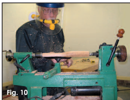
Fig. 10 Turn the handle from a piece of 1-1/4" (5/4) oak.
