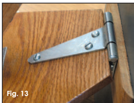
Fig. 13 Bend the hinge to a 30° angle so it fits part "B."
