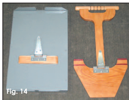
Fig. 14 Mount the hinge in the center of "C."
