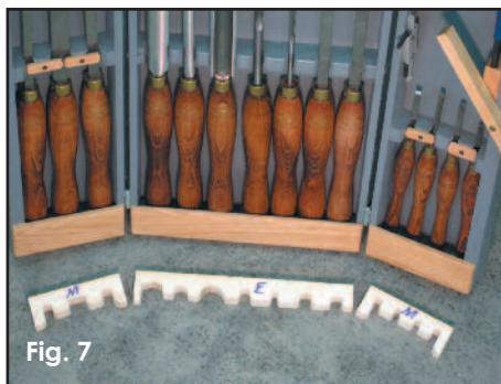
Fig. 7 Trim the tail on the right side of part "E" and leave the others long.
